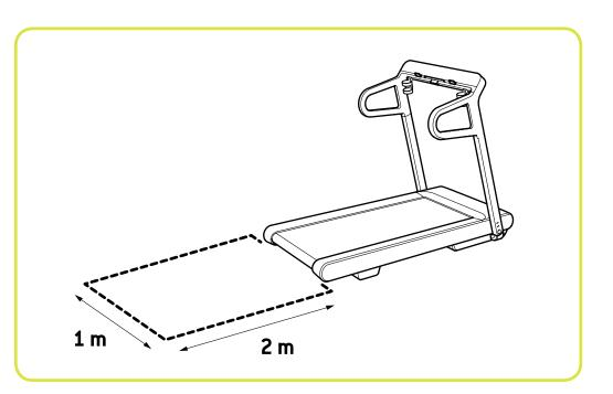
The place of installation must comply with all the suitability requirements laid down in current legislation on this matter. Do not expose the equipment to direct sunlight.
